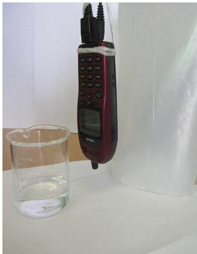
Fig. 7. The process of exposing two water samples to the MP radiation. One of the glasses is wrapped by thin ( 40\mu\text{m} ) four-layered PF. The exposure duration is 1.5 hour.
